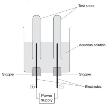
Hydrogen was produced at the negative electrode and oxygen was produced at the positive electrode.
